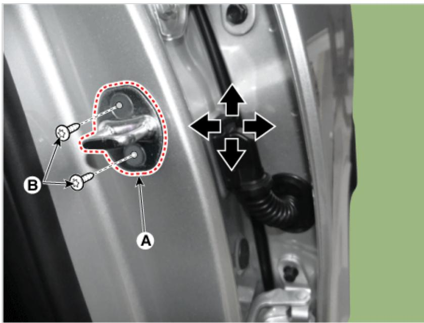
2. Tap on the striker with a plastic hammer to adjust the striker. The striker will not move much, but will give some adjustment.
