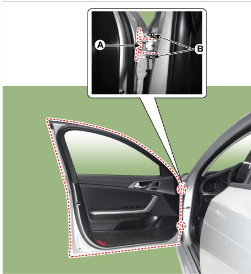
4. Grease the pivot portions of the hinges indicated.
